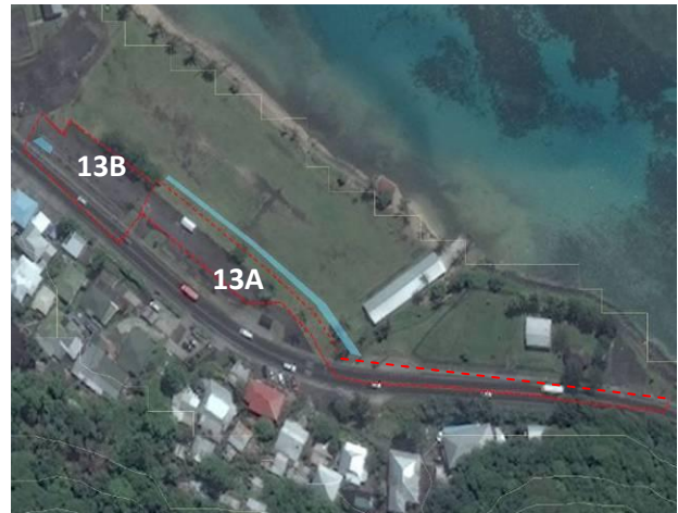
Map depicting retrofit locations (blue polygons) and drainage areas to each site (red dashed line).
