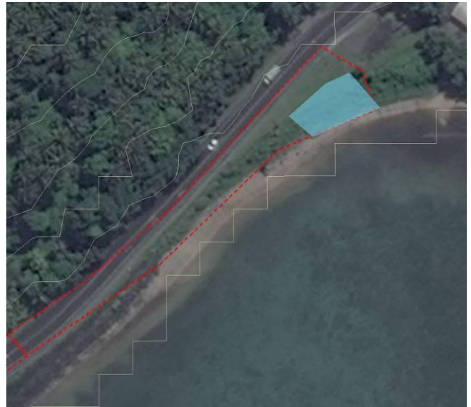
Map depicting the location of proposed bioretention (blue) and area draining to it (red line).
