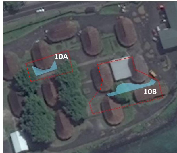
Map depicting location of proposed retrofit (blue polygon) and estimated drainage area (red dashed line).
