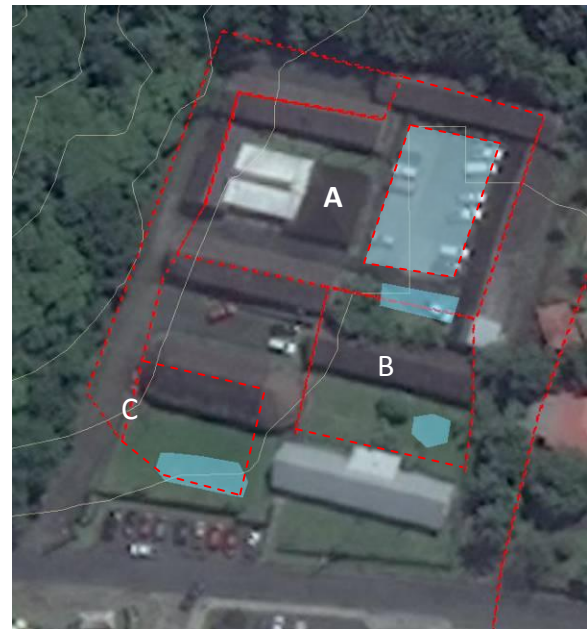
Map showing proposed practice locations (blue) and the areas draining to them (red line).
