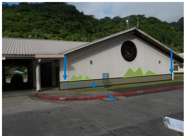
Figure 4F. Location of potential planter boxes to enhance aesthetics of the chapel and reduce runoff contribution from rooftop. Overflow can tie into existing drain near adjacent downspout or at sidewalk.
