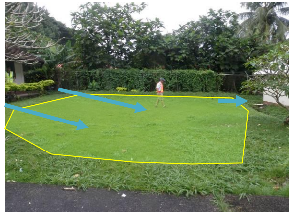
Figure 7A. Proposed location for small bioretention in upper parking lot. A portion of the parking lot is also proposed to be converted to permeable pavers.
