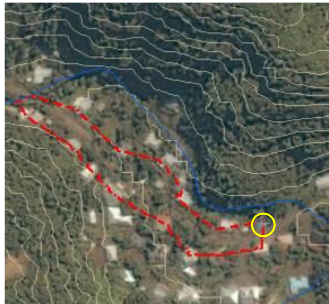
Map showing location of proposed bioretention (blue polygon in yellow circle) and drainage area to practice (red dotted line).
