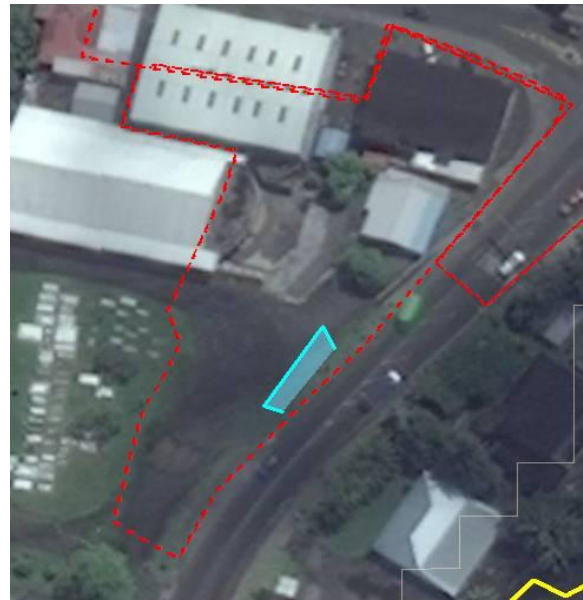
Map showing location of proposed dry swale (blue polygon) and drainage area to practice (red dotted line).
