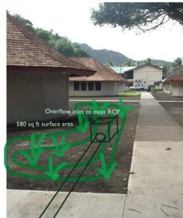
Figure 10A. Looking east at 13-A bioretention cell locations (potential installations on both sides of sidewalk) and partial view of contributing drainage area.
