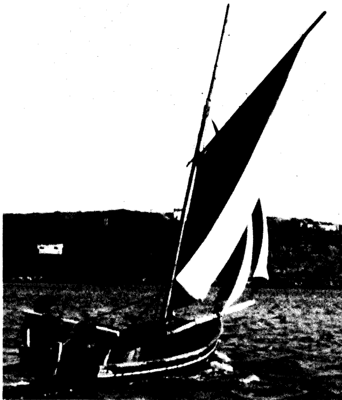
Fig. 2. Gaff rig as a replacement for lateen rig on a traditional Mashua
