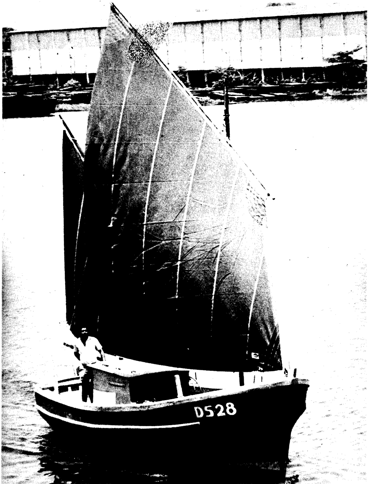
D.S. 28 - Sail-assisted mechanized fishing boat introduced by the Sri Lanka Ministry of Fisheries in early 1983
