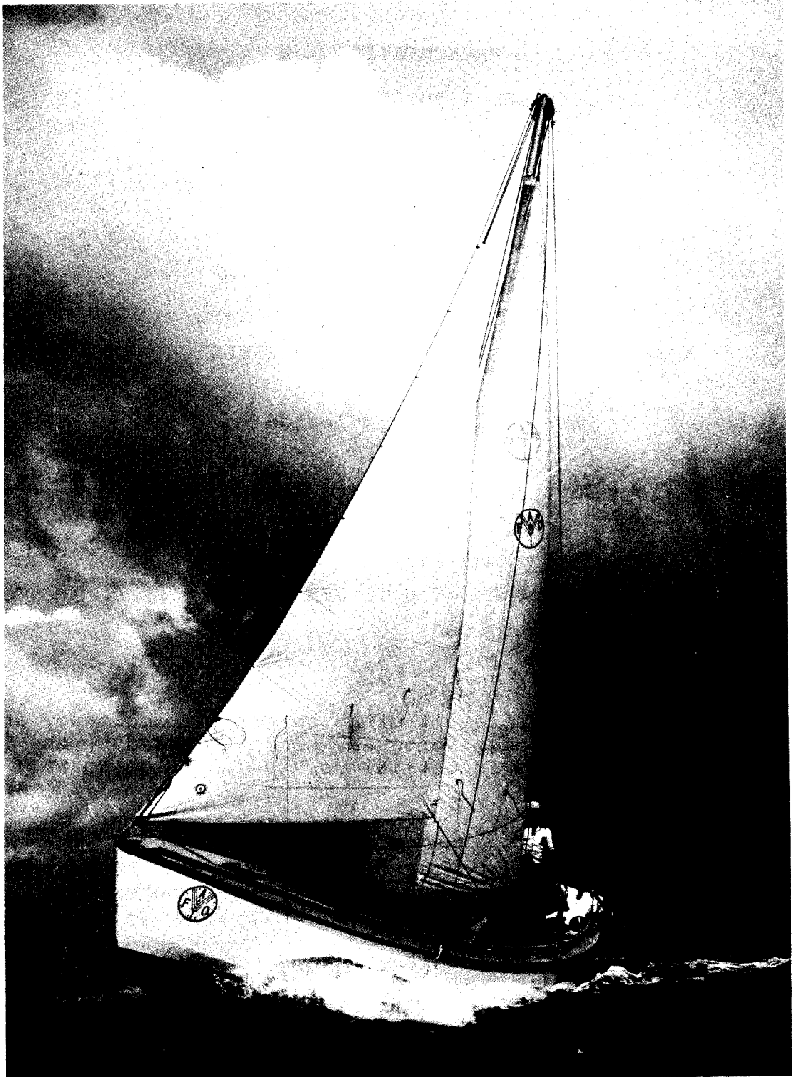
SRL 11 - Sail-assisted mechanized boat introduced by the F.A.O. Bay of Bengal Project, Sri Lanka in 1981
