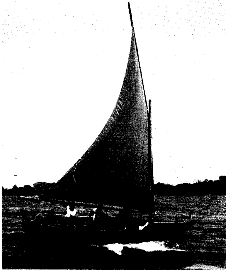
Fig. 12. 5 m (17 ft) fishing boat using a standing lug on northern Lake Malawi
