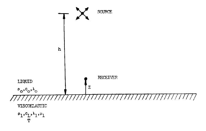
Geometry of Normal Incidence Acoustic Response System: Semi-Infinite Liquid Over a Viscoelastic Halfsrace
