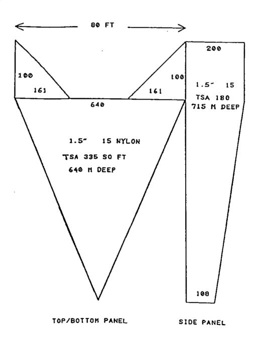
Figure 2. Experimental trawl (Pacific Trawl Co.<sup>©</sup>) used in field tests. TSA = twine surface area; M = meshes; P = mesh cut on point; B = mesh cut on bar (for determining mesh tapers).
