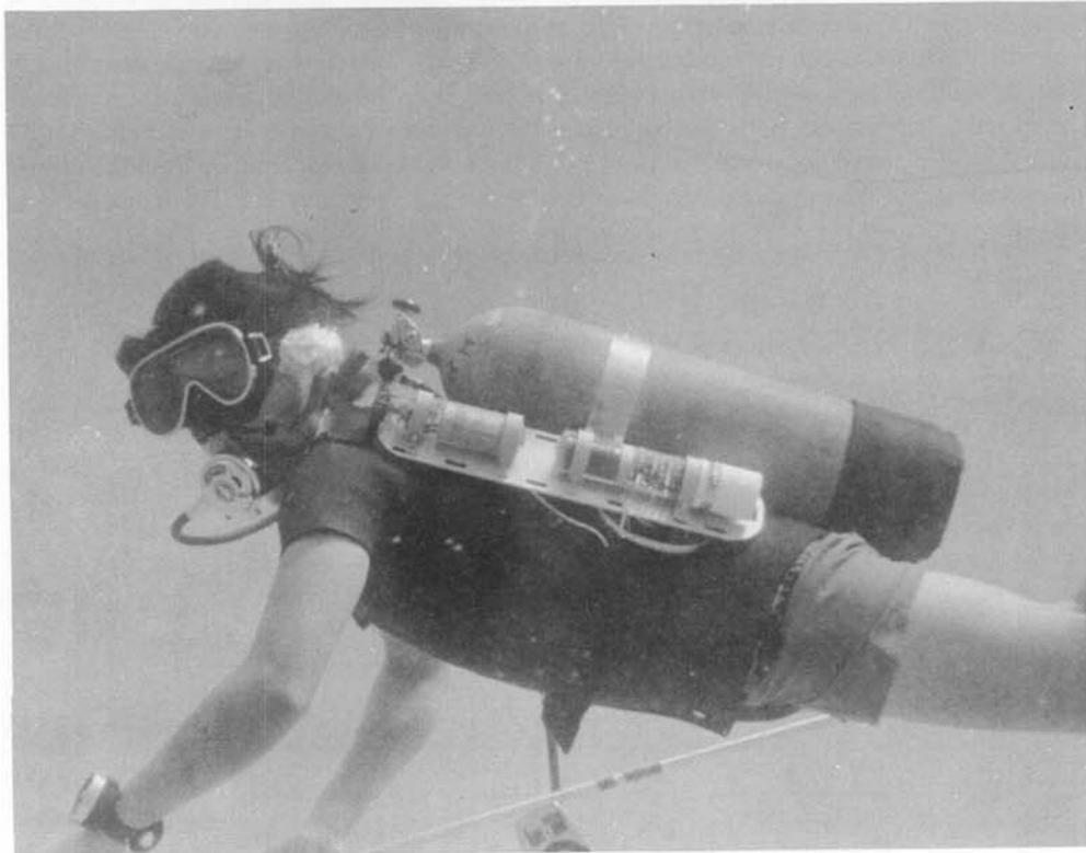
Fig. 6. Underwater photograph showing two separate transmitters alongside the scuba tank.
