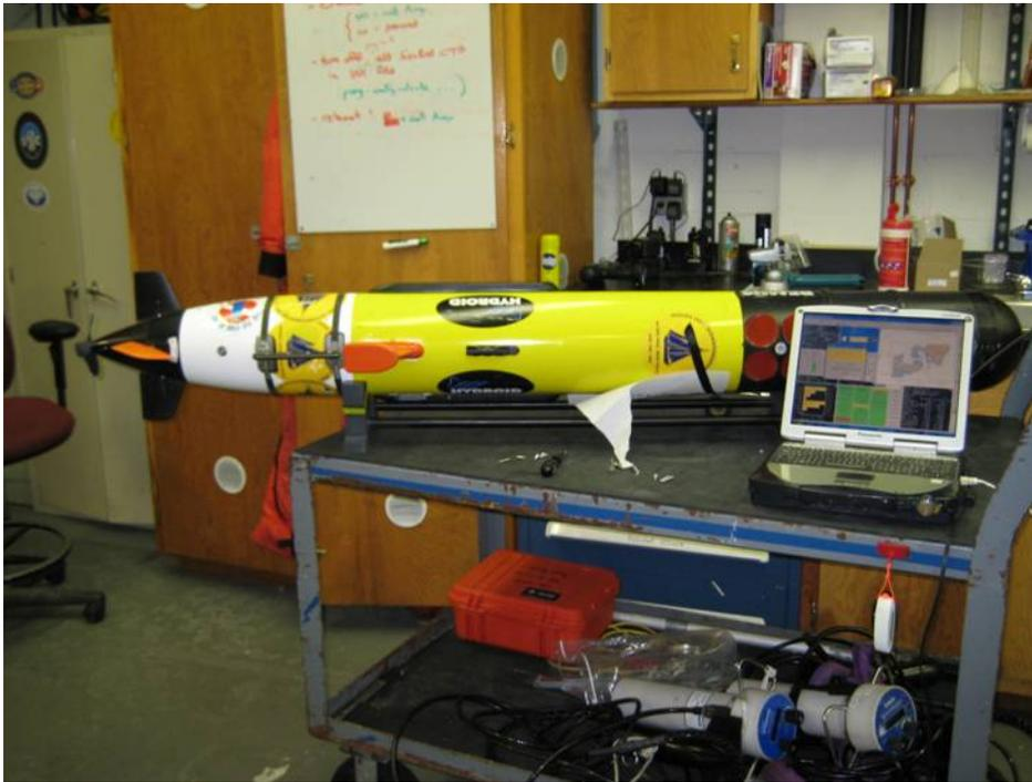
**Figure 16: Picture of the REMUS vehicle and interfacing laptop in the Ocean Systems Laboratory, WHOI.**
