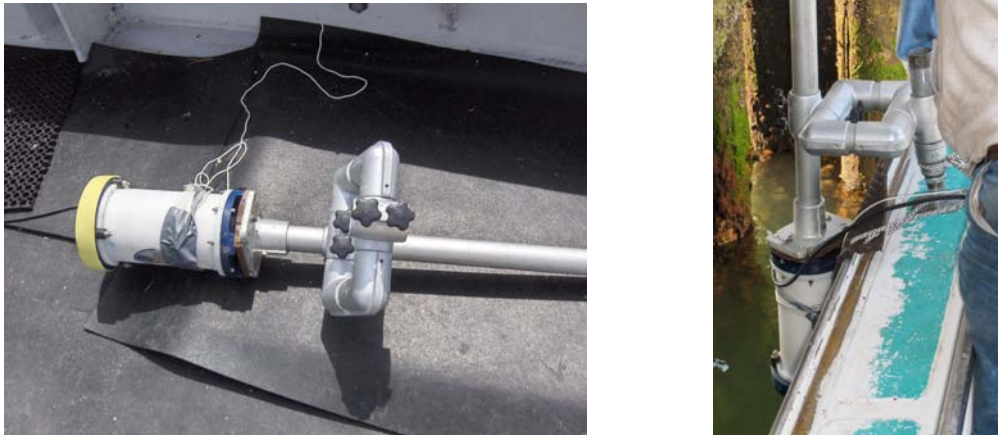
Figure 11 (left) The RDI 300 kHz ADCP mounted on the deployment spar; (right) At each station the downward-looking ADCP was lowered to a depth of about 1.5m.
