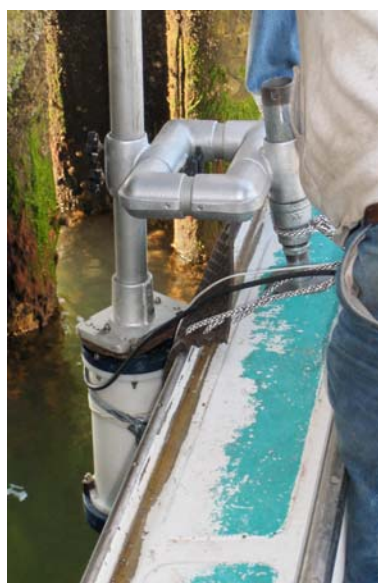
Figure 10 (left) The RDI 300 kHz ADCP mounted on the deployment spar. (right) At each station the downward-looking ADCP was lowered to a depth of about 1.5m.
