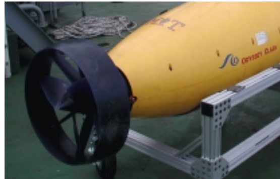
Figure 2: Caribou's ring fin duct thruster
