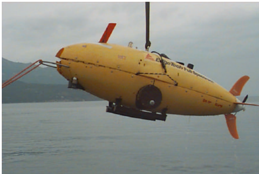
Fig 2. Borealis equipped with the sub-bottom profiler
