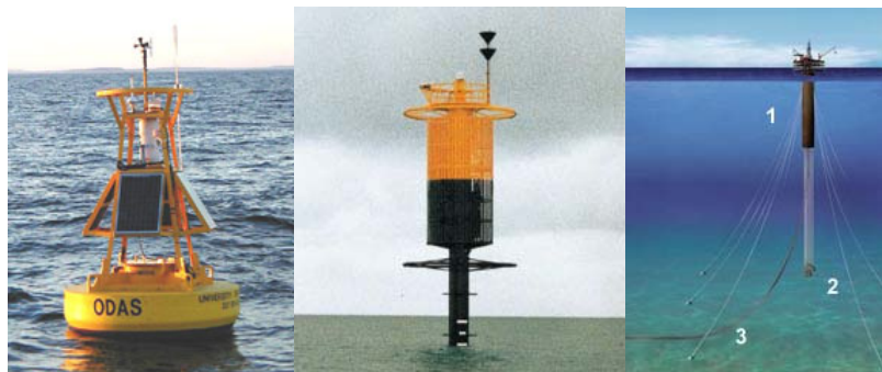
Figure 2. a) Discus Buoy b) Spar Buoy c) DDCV Hoover Diana
