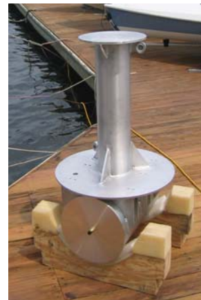
Figure 33. Buoy Assembly: Battery Can and Section 1
