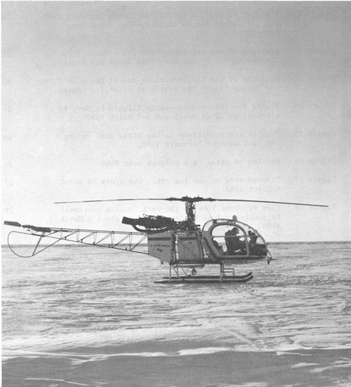
FRONTISPIECE. Alouette II helicopter (belonging to Evergreen Helicopters of Alaska, Inc.), idling at floe site one. The helicopter was equipped with skis, exterior equipment baskets, and rotor with a clutch.
