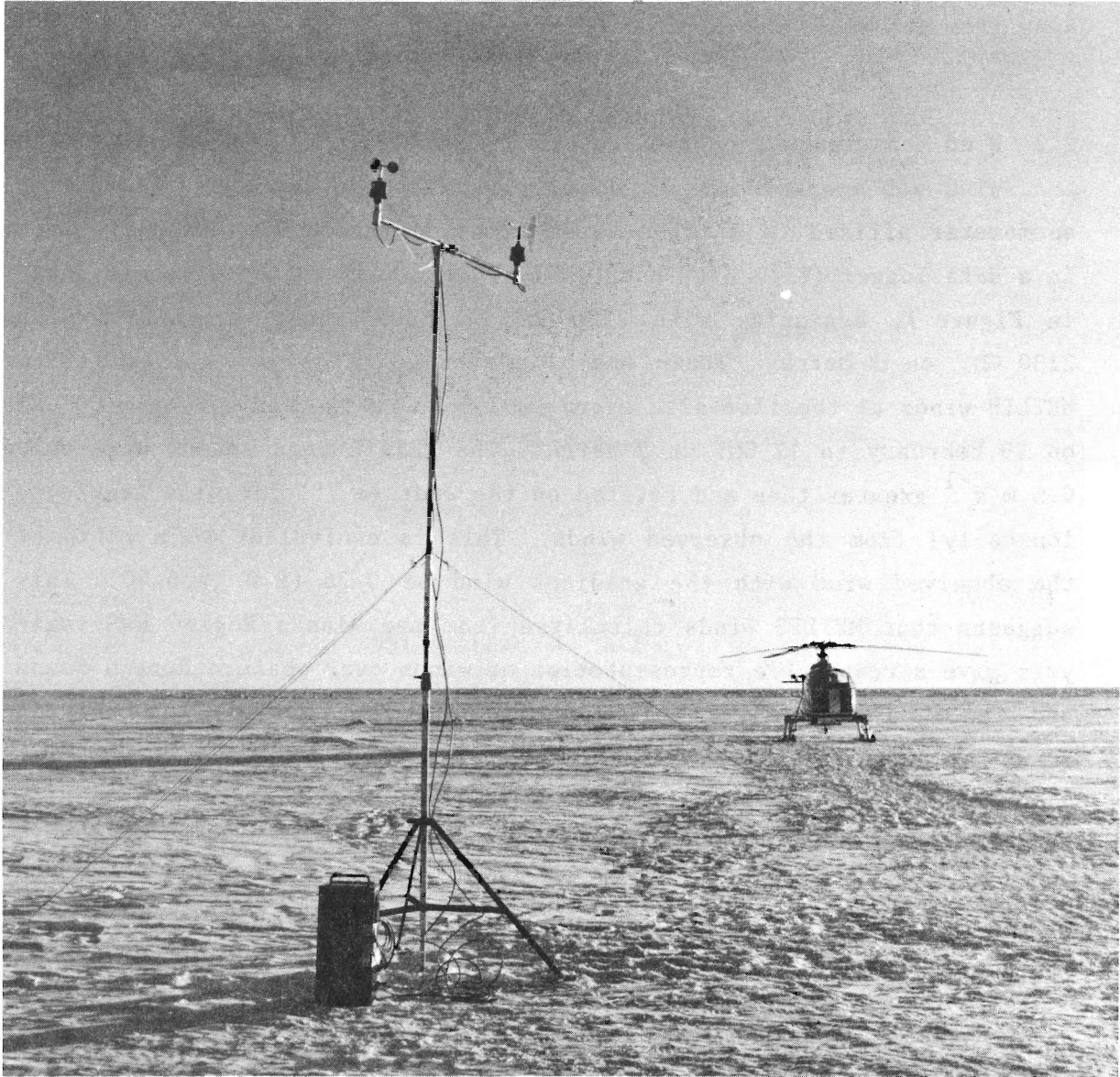
Figure 6. Anemometer with data logger at the first floe site. Cups and vane are 3 m above the surface. Note that helicopter skis, equipment, and footsteps have only penetrated the upper centimeters of the snow. (Photo by D. L. Bell.)
