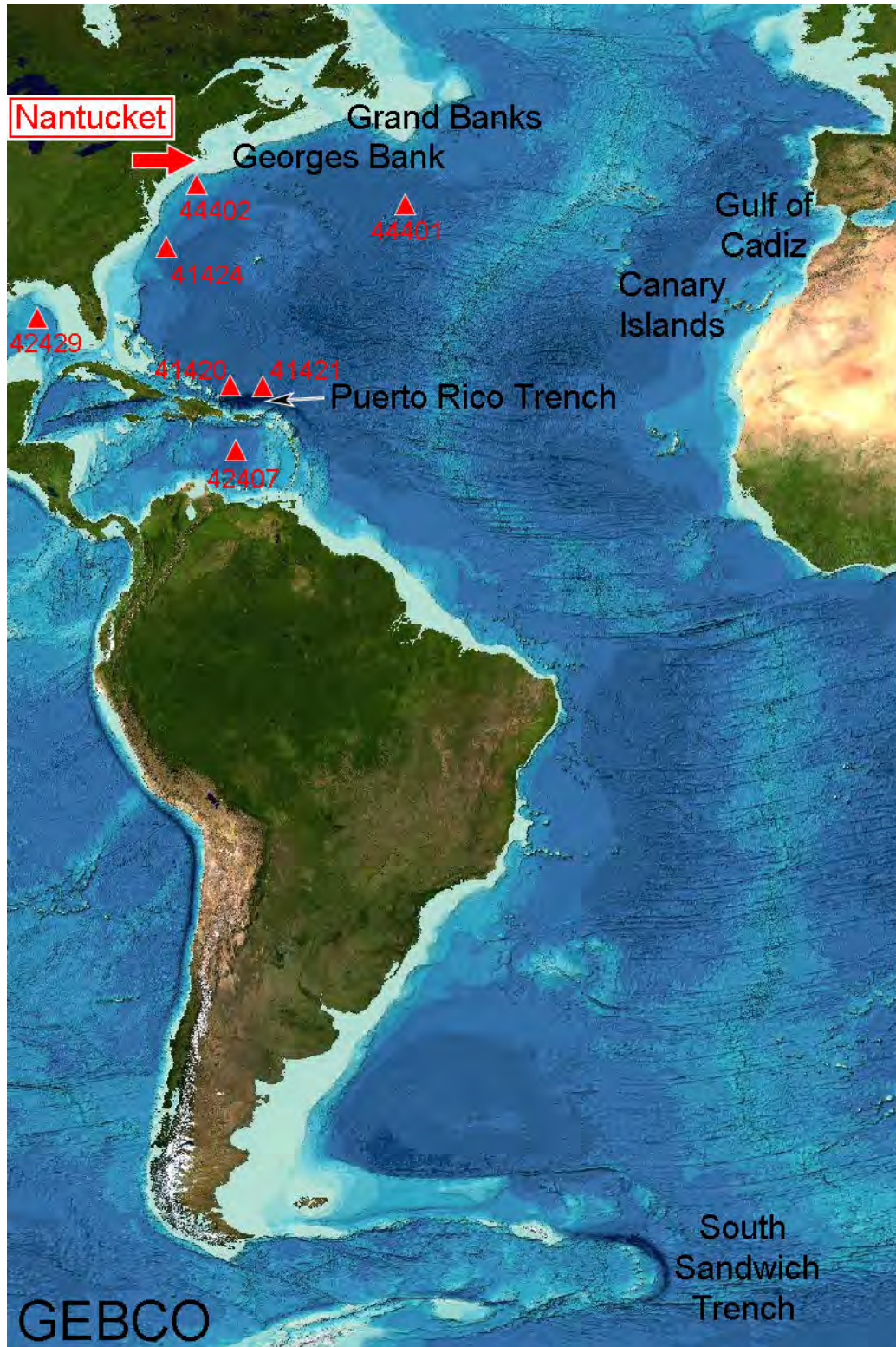
Figure 5: Nantucket’s location in the northwest Atlantic. The underlying chart is based on the GEBCO dataset and is annotated with potential tsunami source areas. Red triangles mark the position of DART® tsunameters that would be assimilated during an event as input to the SIFT forecast system.
