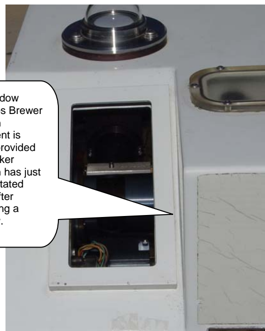
Figure 4-14 Brewer with proper azimuth alignment. No shadow may also indicate azimuth is rotated too far in the counter-clockwise (CCW) direction
