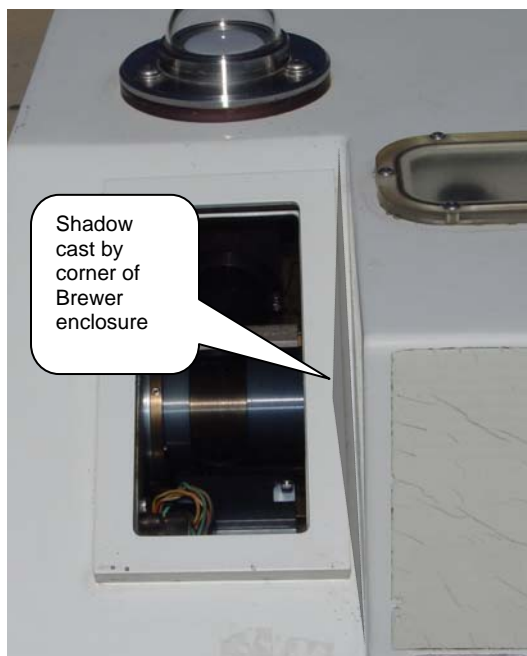
Figure 4-13 Visible shadow caused by Brewer's azimuth alignment being rotated too far in the clockwise (CW) direction
