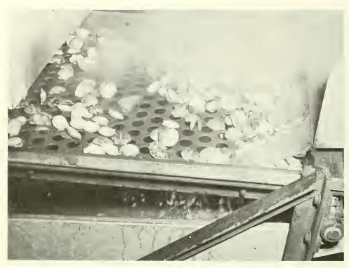
Figure 4.—The vibrating screen containing shells after removal of the meat and viscera to the discharge pipe.
