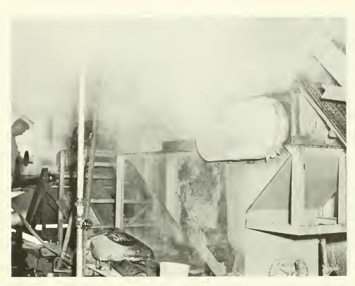
Figure 2.—The shell stock hot water, heat shocking tank with the conveyor for transferring the shell stock to the second set of rotating metal rollers.
