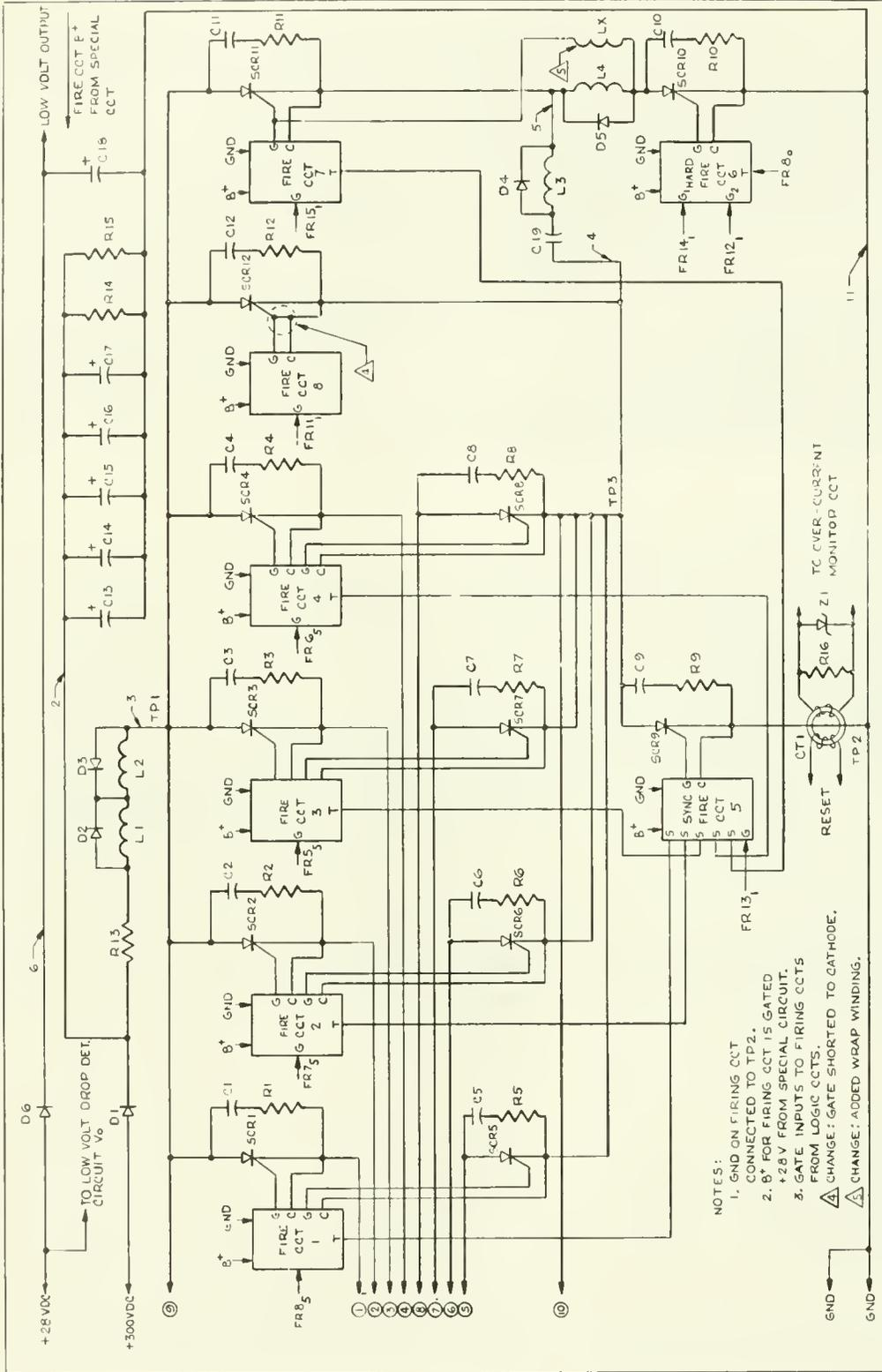
Figure 4. — Electrical schematic of Freshwater Fish Electro-Motivator (FFEM) pulser.
