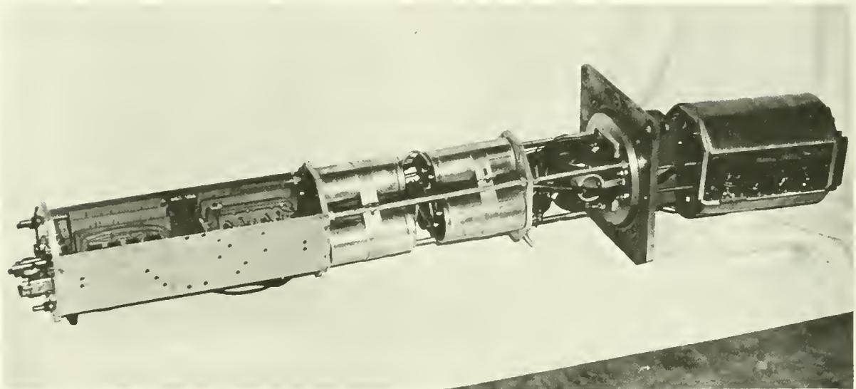
Figure 2. — Freshwater Fish Electro-Motivator (FFEM) pulser with and without protective aluminum housing.
