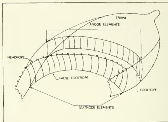
Figure 9. — Diagram of electrical trawl showing arrangement of electrode arrays in mouth of net.
