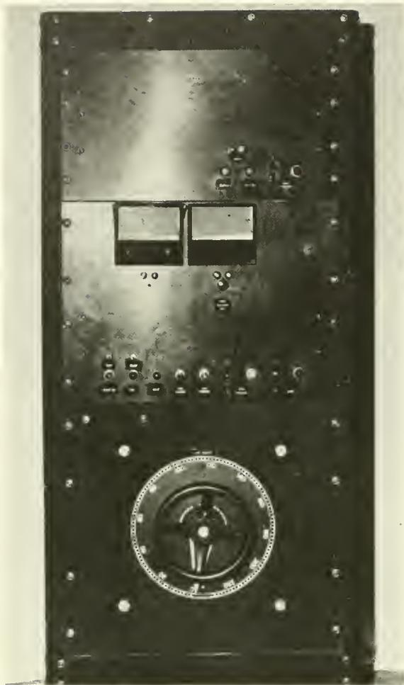
Figure 8. — Freshwater Fish Electro-Motivator (FFEM) power supply.
