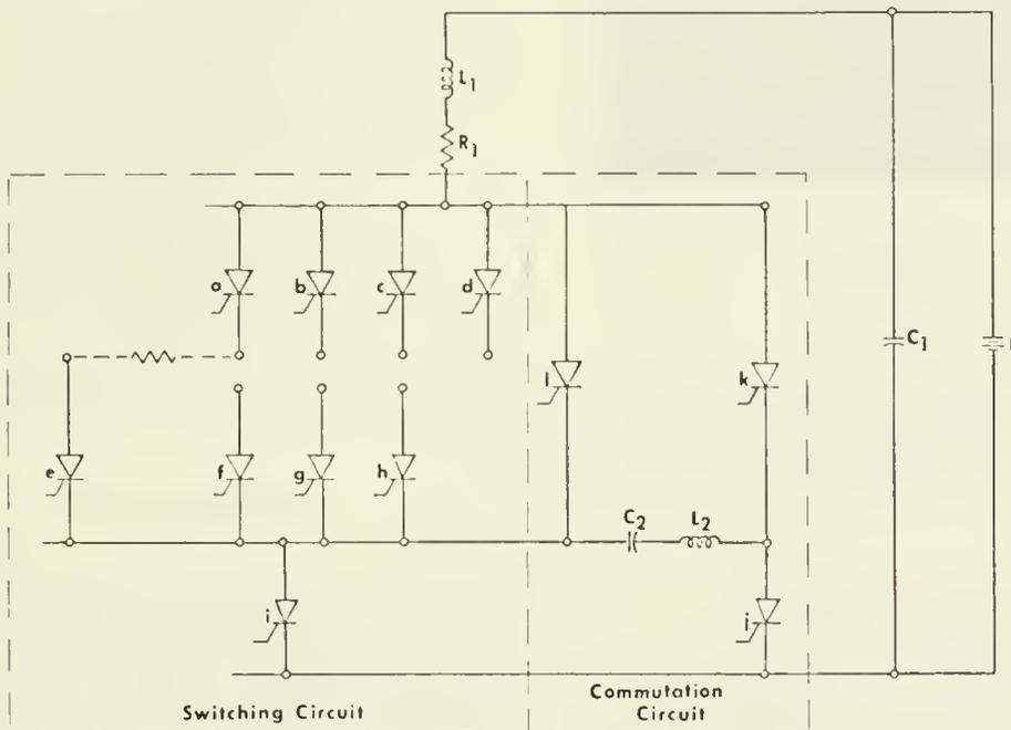
Figure 7. — High power switching and commutation circuit.
