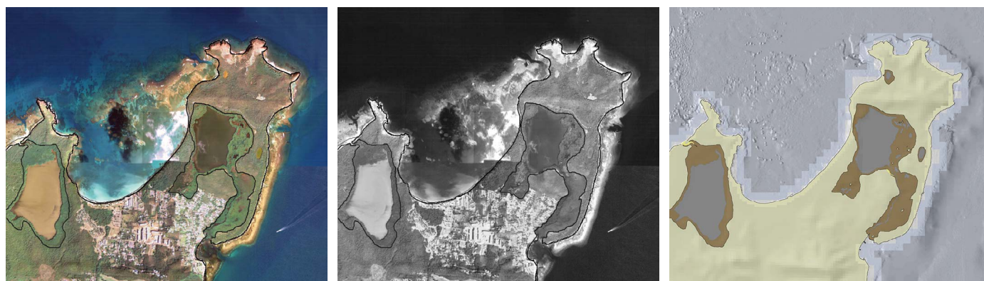
Figure 3.5. Shore complex areas were manually delineated and classified using aerial imagery from 2007 and 2010. (a) Shows the RGB bands, (b) show the Infrared band used to identify mangroves and (c) show the final classified shore complex map in the Las Cabezas de San Juan Nature Reserve area.
