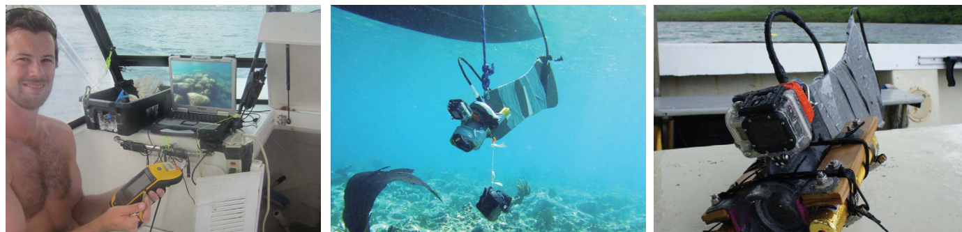
Figure 3.18. (Left) The habitat analyst with field setup: a Toughbook showing live video feed from the drop-camera, and a Trimble GPS to record location and habitat information. (Middle) Drop-camera system under water, the rope and the cable helped the field team to maneuver the camera system to capture both landscape and downward views of the seafloor. (Right) The SeaViewer camera with a GoPro camera mounted on top of the SeaViewer camera, and two lasers positioned in parallel 13 cm apart.
