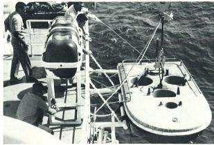
Circulatory surveys by the NOAA ship Ferrel (above, left) use sensors suspended from anchored buoys to measure currents, temperature, and salinity at preselected depths. These data are used to predict tidal currents and to manage pollution in estuarine areas.
