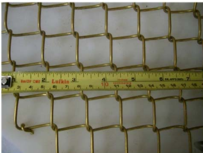
Figure 4. Close-up photograph of the brass mesh net of the CuPod. Source: Kona Blue Water Farms, provided to NMFS in 2011.
