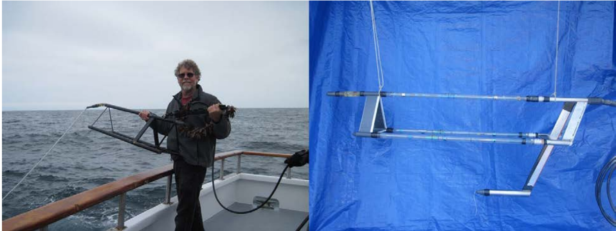
Figure 1.--The volumetric array predecessors included a ‘box-kite’ design that provided three-dimensional localization, but did not perform well at speeds faster than 8 knots.
