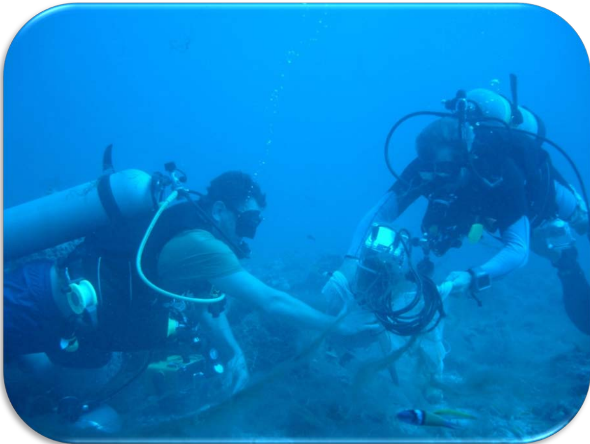
Co-PI Jim Locascio, USF, and Ken Brennan, NMFS Beaufort Laboratory, deploy underwater cameras with hydrophones at selected stations to study acoustics of grouper spawning aggregations. (Photo credit: Mike Judge, NMFS, SEFSC, Miami Laboratory).
