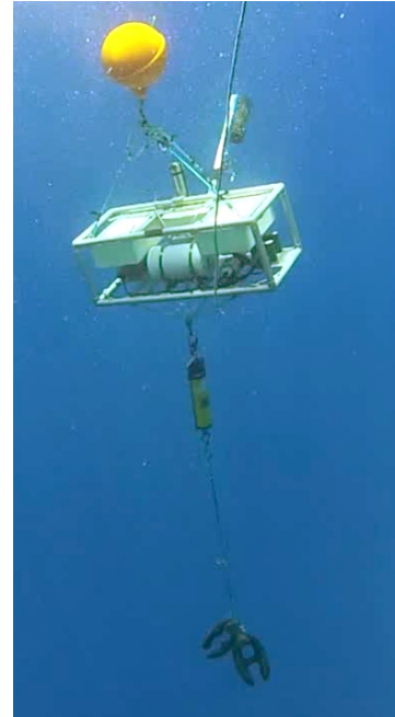
Figure 6.--A BotCam descends from the RV Huki Pono during SE-12-08.
