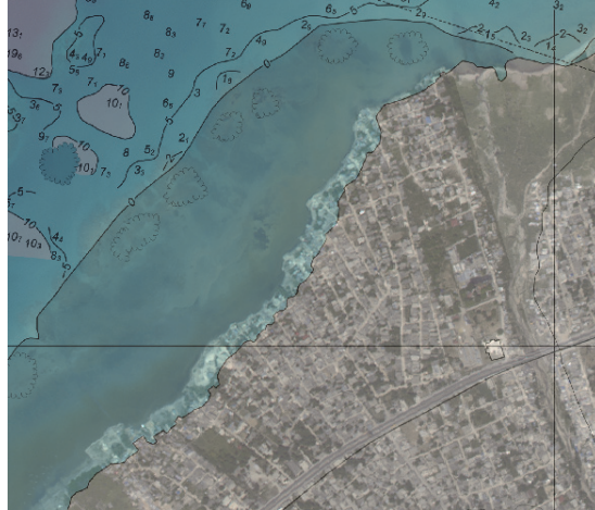
Figure 10. Figure showing the misalignment between WV-2 and the chart.
