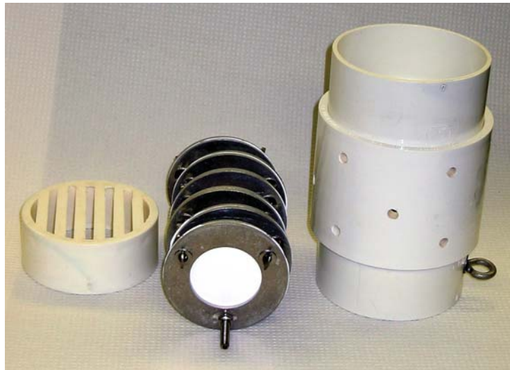
Figure 3. A disassembled POCIS deployment canister with the POCIS disks. Image courtesy of the USGS.
