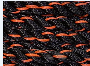
Figure 2.2.1. Example of a color tracer line (orange) woven along the entire length of a black trap line. In the image, the trap line is coiled.
