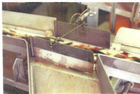
Diverting gates on conveyor
