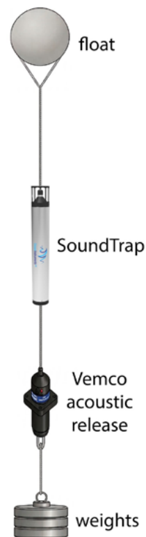
Ocean Instruments NZ SoundTrap recorder mooring. Images are not to scale. Credit: NOAA/NMFS/SEFSC
