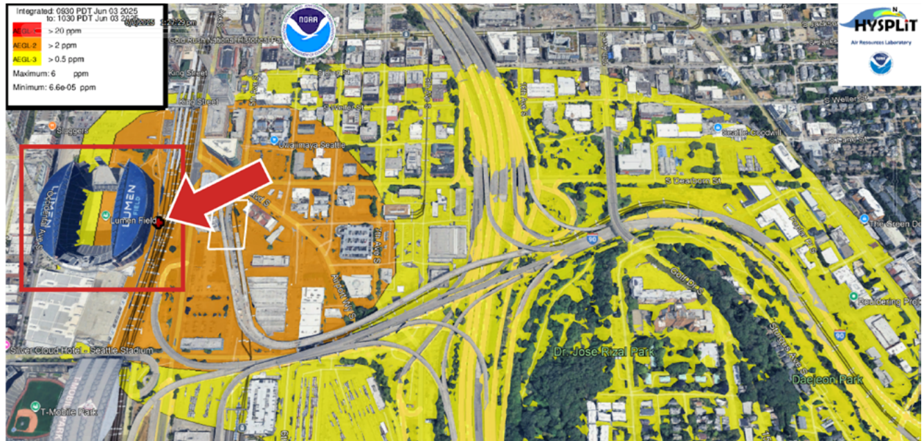
HYSPLIT model forecast of a hypothetical chlorine leak from a rail tanker close to Lumen Field stadium in Seattle, WA. The plume shows the likely direction and dispersion from the site and into the surrounding area. Credit: NOAA/OAR/ARL
