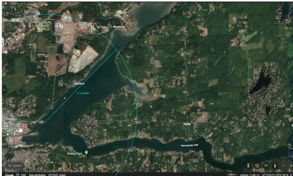
Figure 2. Map showing the lineal extent of the action area resulting from underwater noise (2.12 miles) that would occur from vibratory pile driving (Northwest Environmental Consulting, LLC 2021).
