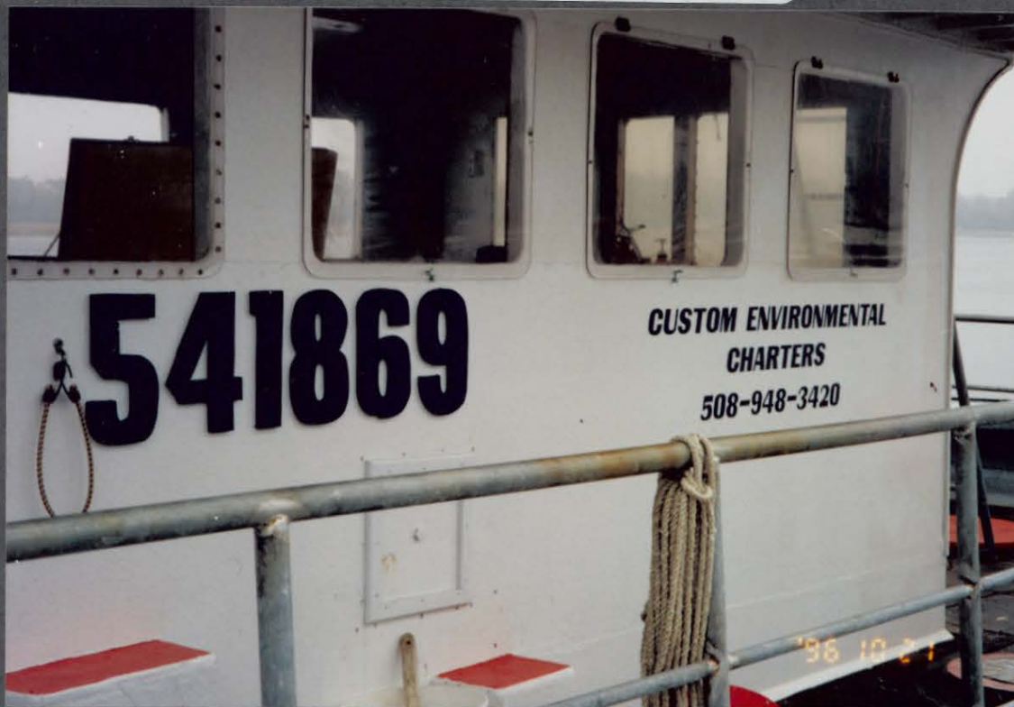
Side view of pilot house. The pilot house was lengthened and enclosed.
