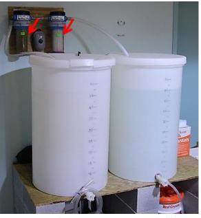
**Figure 5.** Artificial seawater mixing (**left**) and holding (**right**) tanks. After mixing overnight fresh artificial seawater is pumped through 5  $\mu$ m and 0.35  $\mu$ m pleated filters (**arrows**) into the holding tank where it is aerated until use.
