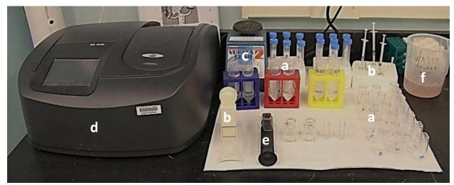
**Figure 20.** A well organized, clean work station will help streamline water quality measurements, reducing time spent and increasing consistency. Within easy reach, the area should include reagents for each test (not shown), testing vials or tubes for each experimental unit (a), volumetric measuring devices (b), a vortex for mixing solutions (c), any special measuring instruments such as a spectrophotometer (d) or refractometer (e), and a waste container (f).
