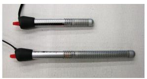
**Figure 17.** Aquarium heaters come in many different sizes and wattages. The smaller 25W heater (**top**) is useful in smaller tanks up to 10 gallons. The larger 200W heater (**bottom**) is suitable for tanks between 50-75 gallons.
