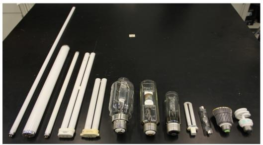
**Figure 8.** Examples of various light bulbs used for coral aquaculture. Left to right: 54 W T5 fluorescent, 20 W T12 fluorescent, 24 W T5 fluorescent, 55 W power compact (PC) fluorescent, 26 W PC fluorescent, 1000 W metal halide, 400 W metal halide, 250 W metal halide, 9 W PC fluorescent, 150 W metal halide, 12 W LED, 5 W compact fluorescent (CFL).
