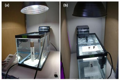
**Figure 41. a)** Each light is standardized to 100  $\mu$ mol/m<sup>2</sup>/s using an LI-192 underwater light sensor (LI-COR®) mounted on a PVC stand (L). **b**) The single coral fragment (F) is centered in the middle of the tank directly under the light source at a specific height on a PVC stand (S).
