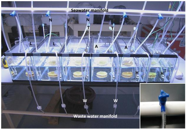
**Figure 38.** Front view of biological dosing setup. Each tank is equipped with a thermometer (**T**), heater (**H**), air line (**A**), new ASW line (**N**), waste water siphon tube (**W**), and a clear lid (**L**). (**inset**) Closeup of plastic needle valve that regulates air and new ASW.
