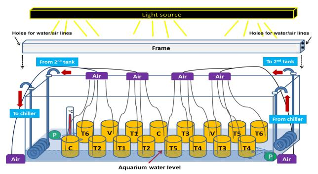
Figure 43. Schematic overview of chemical dosing system. Schematic designed by Lisa May.
