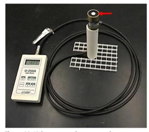
Figure 11. Light meter and sensor used to measure photosynthetically active radiation directly above the sensor (arrow). The sensor has been positioned on a stand constructed from PVC pipe and plastic egg crate material to keep the sensor stable and at a specific height in the water column.
