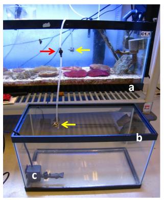
**Figure 21.** Simple drip acclimation setup. Seawater is slowly siphoned from the holding tank (**a**) to the temporary acclimation tank (**b**) through air-line tubing. A small ball valve (**red arrow**) regulates flow rate and stainless steel clamps (**yellow arrows**) keep the tubing in place. Water is circulated by a small powerhead (**c**).
