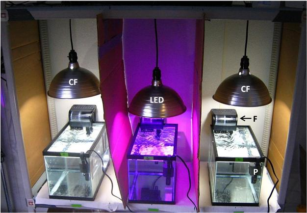
**Figure 40.** Overview of light experimental setup. Each replicate has its own light source (**CF** or **LED**), BIO-Wheel<sup>®</sup> powerfilter (**F**) and small powerhead (**P**) and are separated by cardboard and black plastic sheeting (not shown) to reduce stray light. Only three of the six replicates are shown here.
