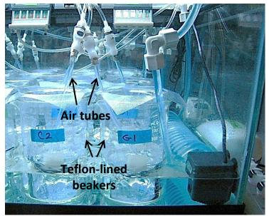
Figure 45. Each replicate consists of a Teflon<sup>®</sup>-lined beaker and a single Teflon<sup>®</sup> air tube.
