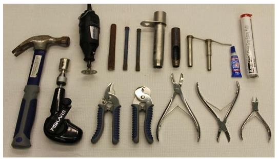
**Figure 32.** Examples of tools used for fragmenting coral. They include a hammer, a hand drill fitted with a hole saw, a Dremel<sup>®</sup> rotary tool, various sizes of chisels and corers or leather punches, "coral clippers" similar to pruning shears or bone cutters, and adhesives.
