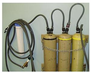
**Figure 3.** Mixed bed deionizing system for preparing artifical seawater. Tap water passes through a 1  $\mu$ m pre-filter (**white cylinder**), an activated carbon tank (**black band**), and then through the mixed bed working and polishing deionizer tanks (**yellow bands**). A light indicates when the working tank is spent.
