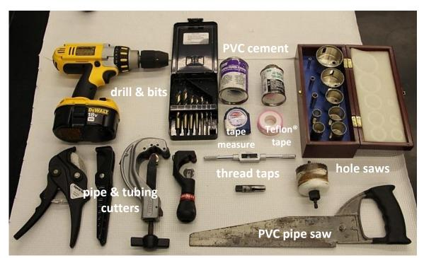
**Figure 13.** Tools typically needed to construct experimental setups. Most can be found at the local hardware store. Some like diamond-coated hole saws and plastic-specific drill bits may need to be ordered (e.g., www.mcmaster.com). Other tools sometimes used but not shown here are a circular saw (for cutting acrylic sheets or wood) and a Dremel<sup>®</sup> rotary tool (for cutting, grinding, and sanding).
