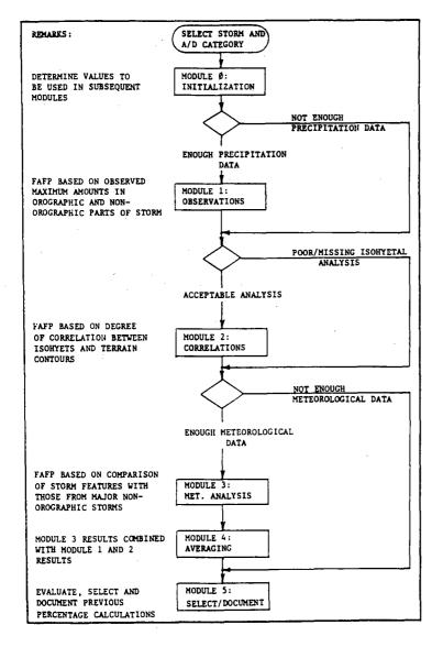
Figure 7.2. -- Main flowchart for SSM.
