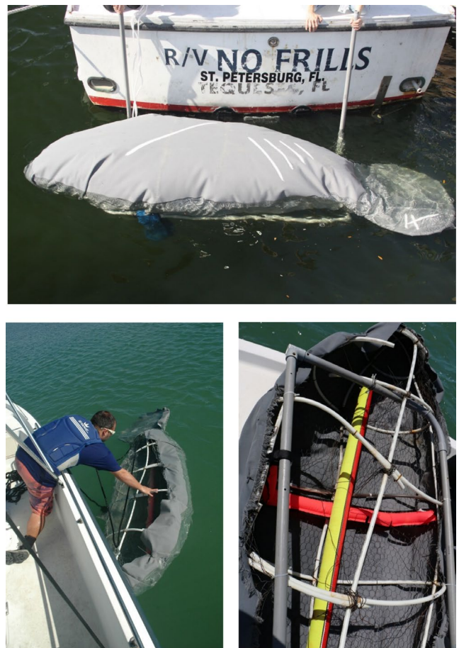
FIGURE 1 | A replica of a Florida manatee, constructed with chicken wire (poultry netting), was used to measure the probability of detecting a manatee under different environmental conditions. Dive weights (top photo) and the yellow/red inflatable lift bags can be seen in the photos.
