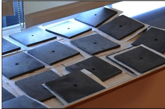
Figure 8. Scraped and rinsed CAU plates cooling on paper trays.
