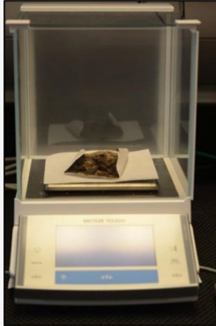
Figure 11. Weighing filter paper.
