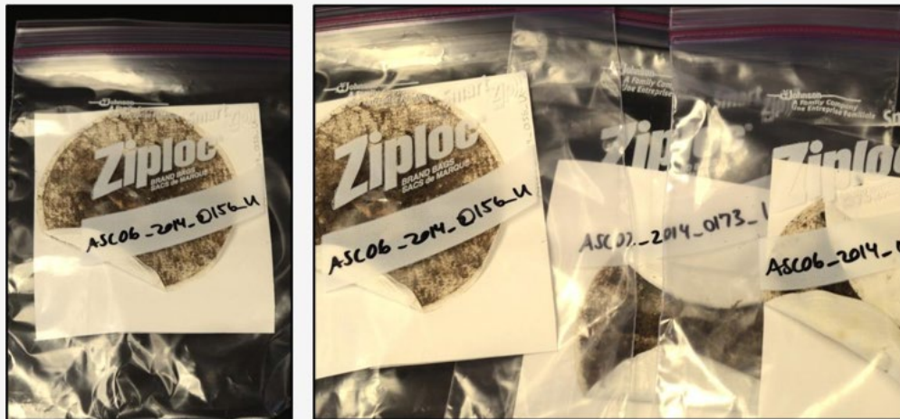
Figure 12. Filter papers stored in labeled plastic bags for archiving.
