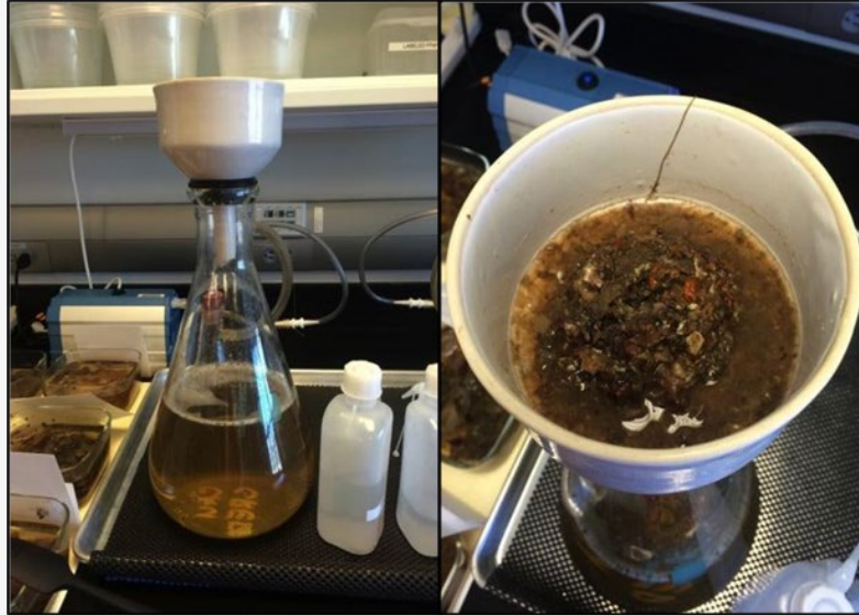
Figure 9. Vacuum filtration of fleshy material using Buchner funnel.
