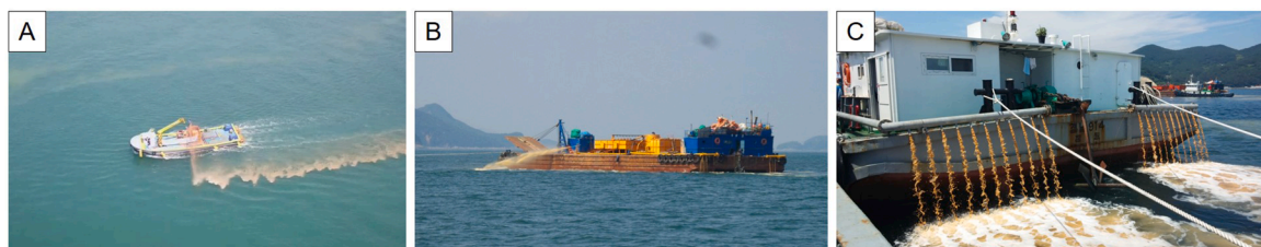
Fig. 11. Various methods of clay dispersion for HAB removal in Korea. (A) 2 G clay dispenser; (B) 3 G clay dispenser; (C) Spraying modified clay.
