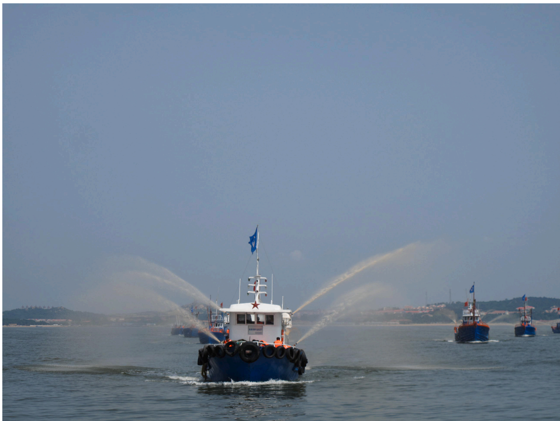
Fig. 13. Large scale HAB suppression using marine clay in open (oceanic) waters in China.
