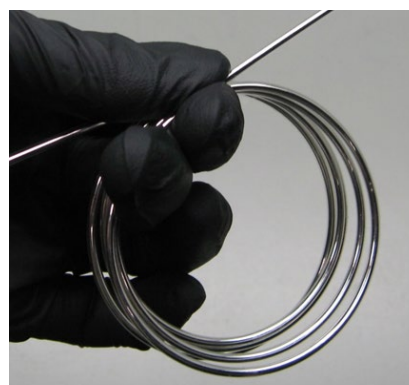
Figure 4. Picture of hollow fiber produced using a relatively large internal diameter (ID = 1500 \mu\text{m} ) plastic capillary.
