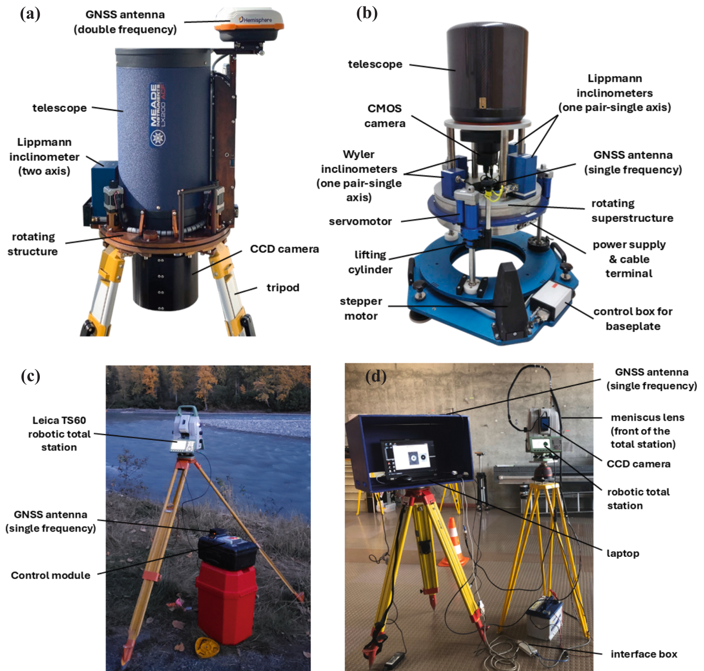
Fig. 2. Design features of (a) VESTA, (b) CODIAC, (c) TSACS, and (d) QDaedalus systems.
