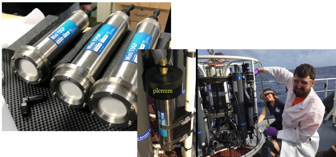
Figure 1. A photograph of three newly developed fast response GTDs (upper right) developed for this project and a photograph of the new sensor being used on the ship's CTD (lower right).
