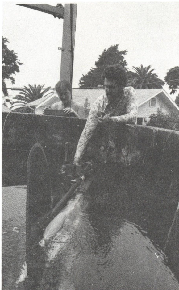
Micro-Patch Sampler is immersed in the Deep Tank by Brown while Carol Kimbrell takes observations. The messenger weights above the trigger actuate the sampler to close sample bottles and open and close the nets at depth.
