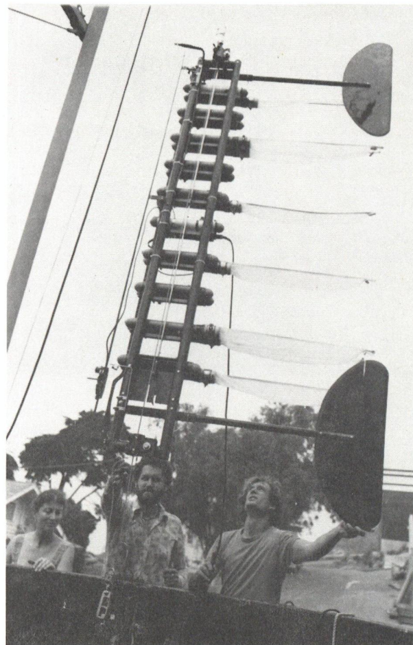
Lee Inness-Brown, Technician, rigs actuation weights on Micro-Patch Sampler as Carol Kimbrell and Dr. Robert Owen watch. Note the close spacing between the sampling tubes. The trolley-mounted thermistor used for temperature microprofile is visible at the lower left side of the MPS frame.
