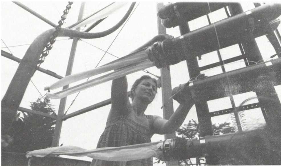
Fishery Biologist Carol Kimbrell inserts paired plankton nets on Micro-Patch Sampler (MPS) prepared for statis testing in the Deep Tank Facility of the Scripps Institution of Oceanography.
