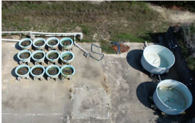
Figure 1. Experimental set up of 296 L tanks ( n = 12 , left) with floating treatment wetlands installed, and the mixing tanks ( n = 2 , right) for dilution of brackish water pumped from the adjacent estuary to attain the three salinity levels ( 0.5 , 5.0 , and 18 \text{ g}\cdot\text{L}^{-1} ).
