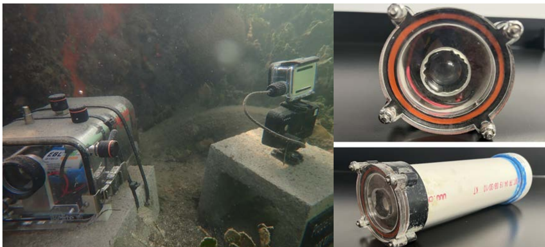
Figure 5. Left: Infrared emitter in Ikelite camera housing. Right: Infrared emitter in custom-built PVC and acrylic enclosure.
