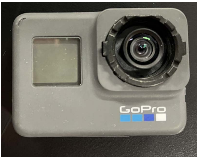
Figure 4. Left: GoPro HERO6 with infrared lens. Right: Pseudodiploria strigosa colony illuminated by infrared light during time lapse deployment.
