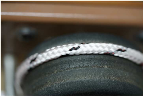
Figure 1. Nautilus-developed capacitive strain-sensing rope
