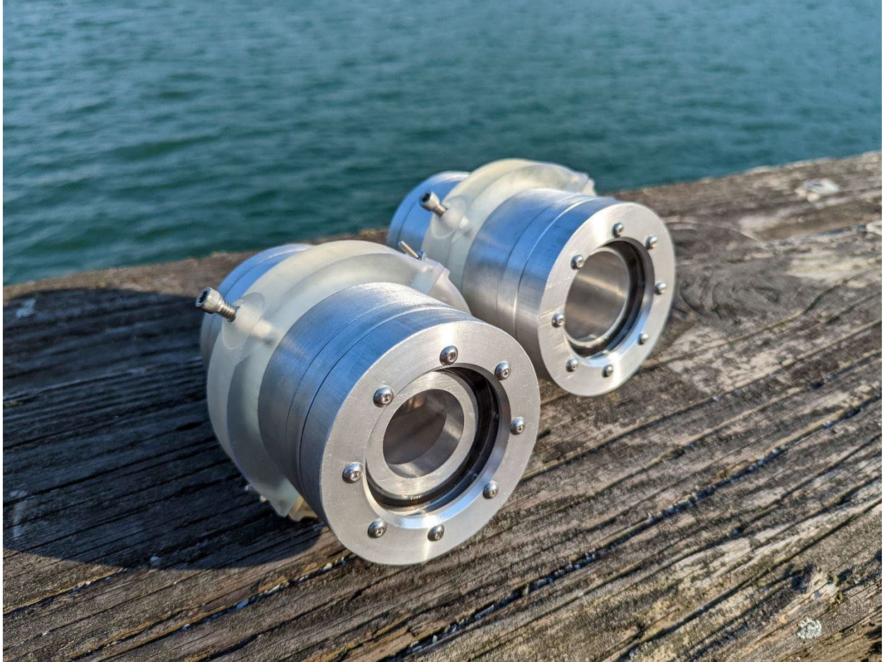
Figure 27. -- Deepwater camera and lighting housings produced at Oregon State University's Innovation Lab. Depth ratings for the housings exceed 1,000 m.
