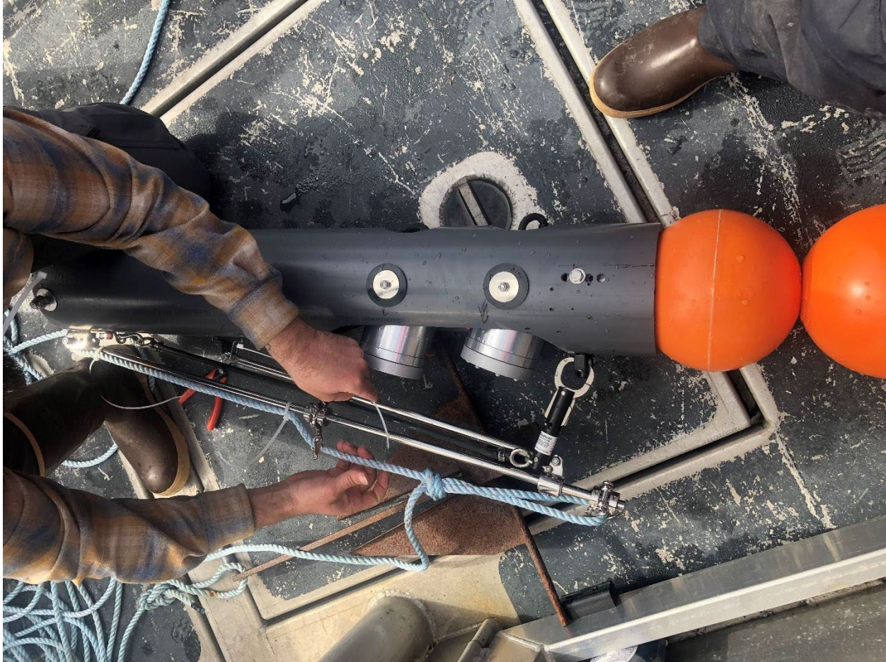
Figure 28. -- Deepwater BICS-type camera system attached to groundline and ready for test deployment. The system is designed to be attached inline on longline gear and will record imagery of the gear actively fishing and interacting with seafloor biota.
