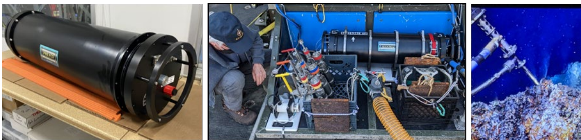
Figure 1. In this project we produced an in-situ methane analyzer, which was deployed on the Jason ROV and used to measure methane from deep sea hydrothermal vents.
