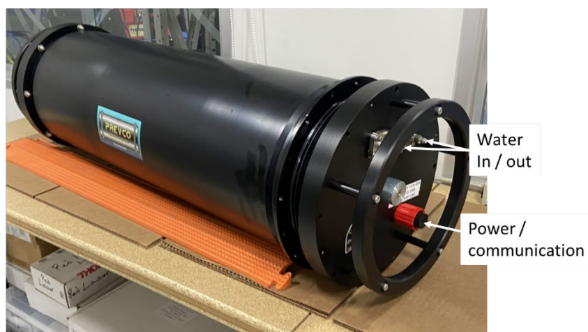
Figure 4. Picture of underwater housing designed and built for the CAS, alongside a list of specifications.
