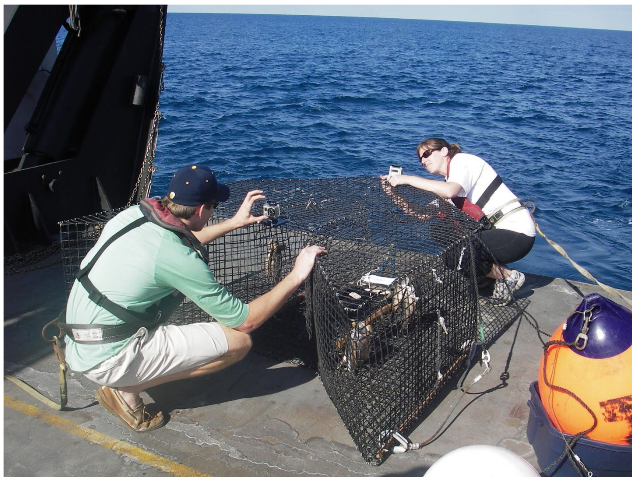
Fig. 1. Baited chevron traps with attached video cameras used by the Southeast Reef Fish Survey between North Carolina and Florida in 2015–2023.
