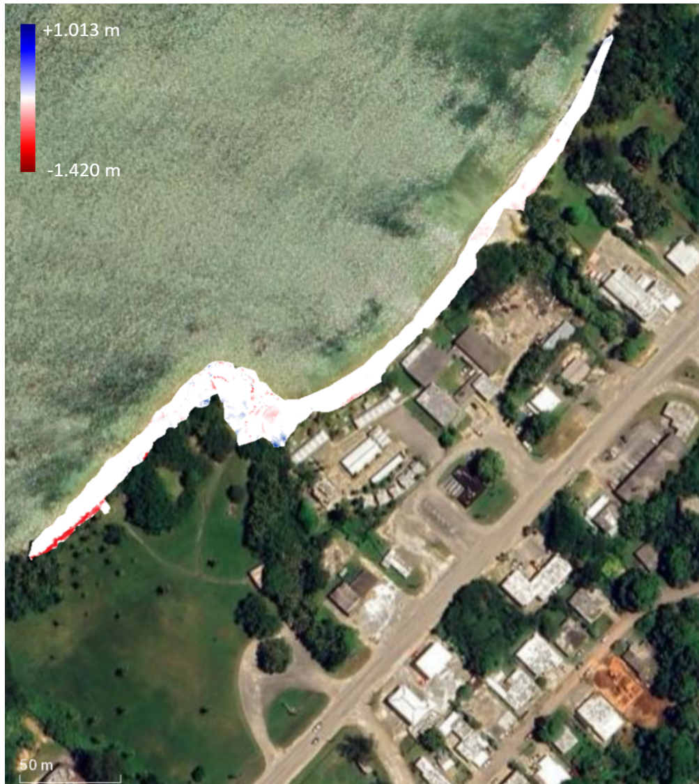
Figure 51. Surface elevation change analysis for Agat unit from February 2023 to July 2023. Positive values (blue) indicate net increase in elevation (accretion) and negative values (red) indicate net decrease (erosion) over the five-month time period. Note these outputs should be interpreted by end-users familiar with the park to discern data artifacts. NPS image.
