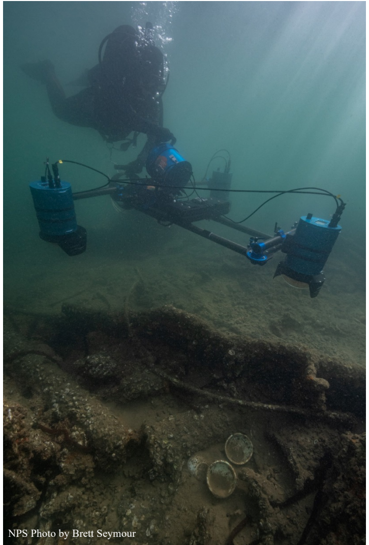
Figure 9: Diver Using DPV mounted 3 camera system called the Sea Array
