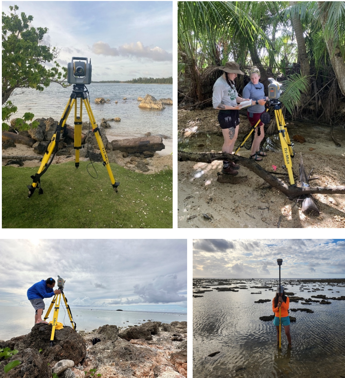
Figure 11. Project team members collecting LiDAR and GNSS data at the Asan Beach and Agat Ga'an Point units.
