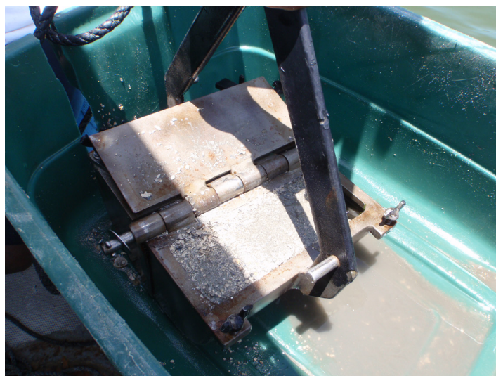
Figure 6. Image of the PONAR grab used to collect sediments in the STXEEMP.
