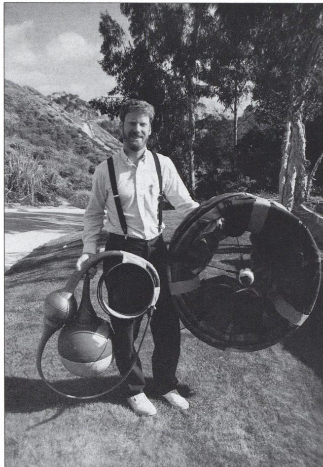
This is the correct holding method for deployment of the standard Global Lagrangian Drifter.
