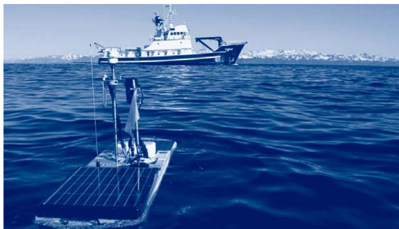
Autonomous glider with sensors. Credit: Evans Wiley, NOAA
