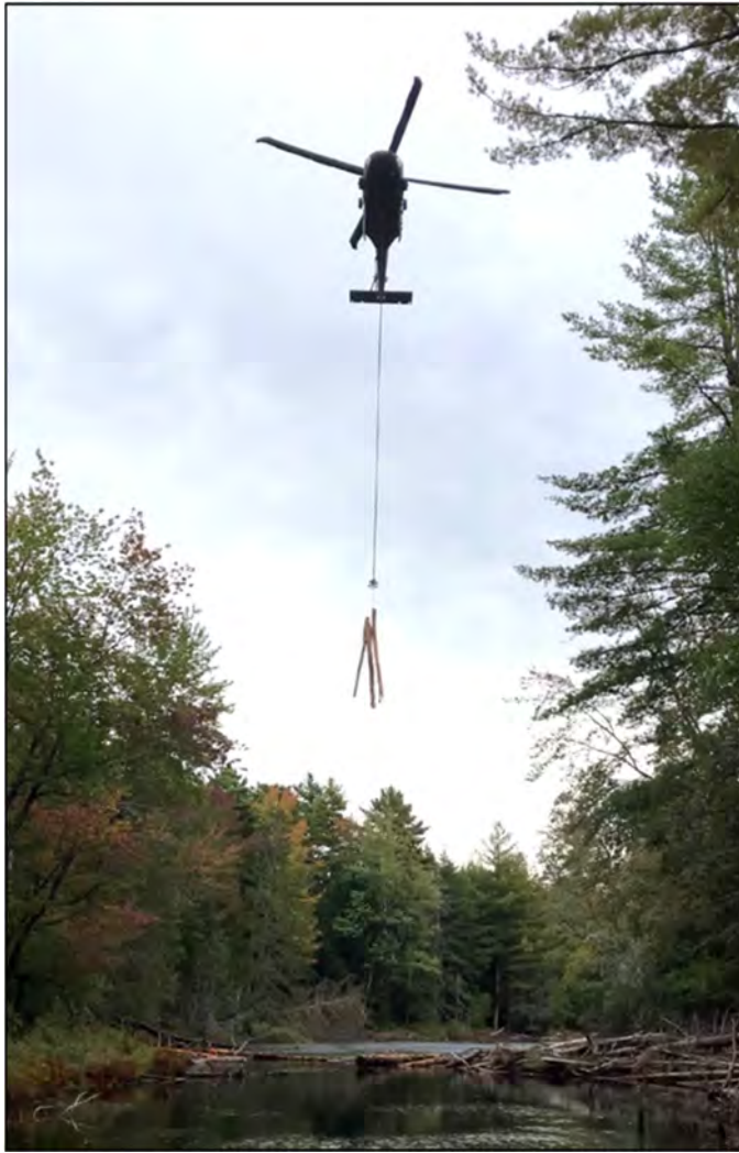
Figure 3.3.3. Maine Army National Guard UH-60 helicopter preparing to drop a load of logs into the Narraguagus River, 2024. Photo Credit: Project SHARE.
