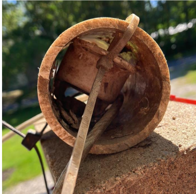
Figure 2: Example of one type of logger housing. ( Photo credit: Danielle Frechette )
