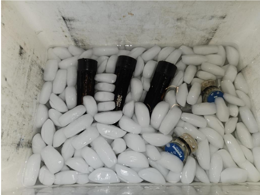
Figure 1: Ice bath example. Note, a mix of water and ice is required—it's difficult to show because the ice floats. Loggers should be submerged, or at a minimum, their sensors should be submerged. (Photo credit: Graham Goulette)
