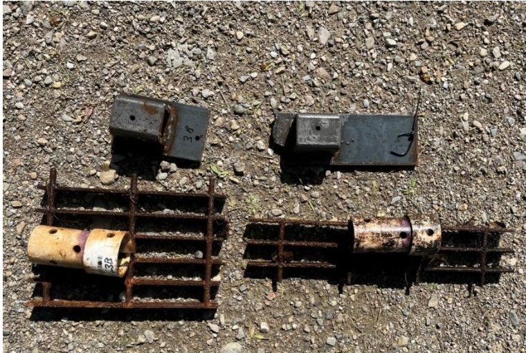
Figure 3: Example of steel housing. Note: the metal chain is not currently attached to the housing units. A 3/8" shackle will attach a chain to the metal bar via the hole opposite the square tube end. (Photo credit: Scott Craig)
